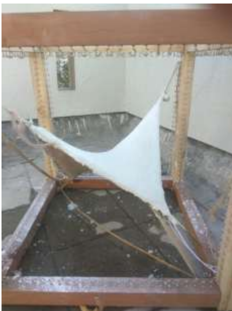
Fig. 70 Applied layer of cement Paster & the layer of cement sand 1:4 mortar layer by layer .
