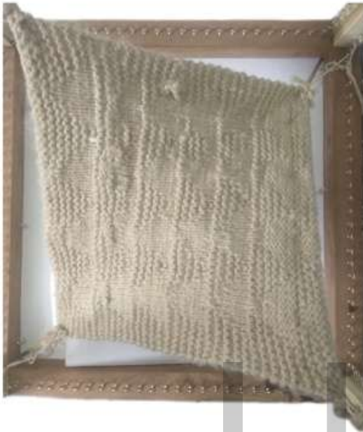
Fig. 68 Plan View Prestressed knitted cloth as stay in place formwork
