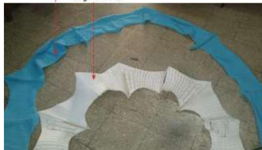
Fig. 87 Unrolled surfaces of paper model and all knitted surfaces joined
