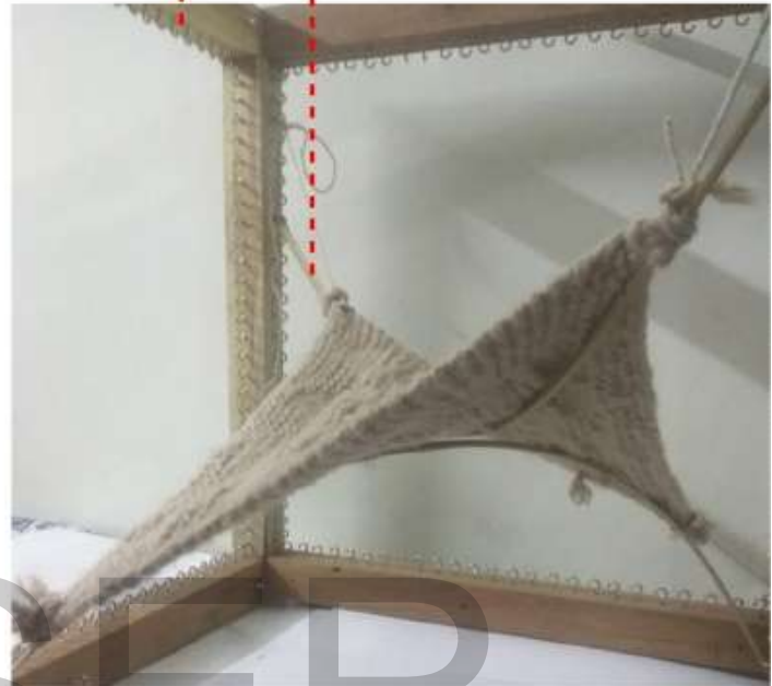
Fig.69 View Prestressed knitted cloth as stay in place formwork
